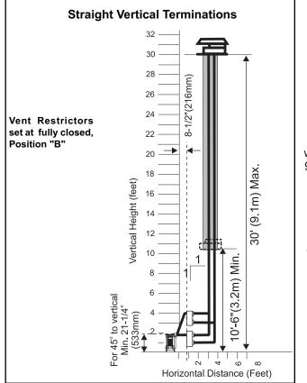
Masonry chimneys may take various contours which the flexible liner will accommodate. However, **keep the flexible liner as straight as possible**, avoid unnecessary bending.
